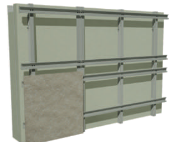
Step 3 Level, lock panel and continue installation of first row of panels
