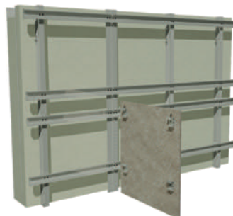
Step 2 MSF standard installation left to right from ground floor upwards
