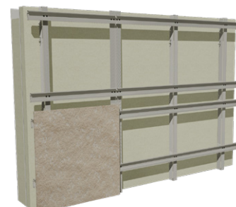
Step 3 Level, lock panel and continue installation of first row of panels
