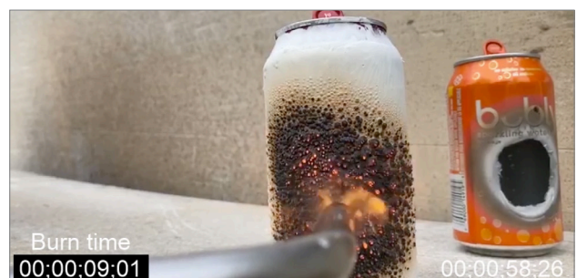
Aluminium can exposed to fire, with and without Zenova FP applied.
